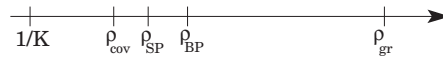
FIG. 5. Sizes of the covering of the hypergraph obtained by the BP, the SP, and the greedy algorithm for a HS problem with L=4 and K=6 , for 12 288 variables and 8192 tests. The COV-UNCOV threshold in this case is equal to \rho_{cov} \approx 0.178 ; the SP algorithm allows us to find solutions of size \rho_{SP} \approx 0.182 ; the BP algorithm generates coverings of size \rho_{BP} \approx 0.186 . Finally, the greedy algorithm gives solutions of size \rho_{gr} \approx 0.212 .
